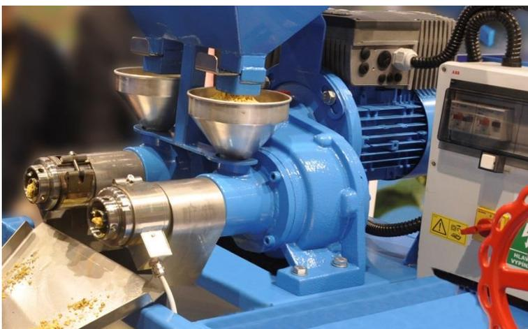
For pressing of these crops, the presses are regularly equipped with a frequency changer of the main drive, which allows optimization of the screw revolutions, depending on the properties of the pressed oilseed. This year we have introduced a new special heat sleeve, which helps maintain a constant temperature in the press chamber, thereby further facilitating the optimization of pressing parameters.
